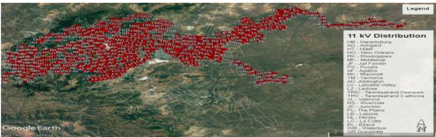
The drawing above indicates the routes of Greater Tzaneen Municipality 11kV overhead lines.
